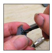
Step 1 - Bore out pivot: Use a 4.5mm bit to bore out the hole where the pivot axle would go.
