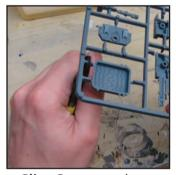
**First Clip:** Cut away the part from the sprue. Leave a small amount of sprue attached.
