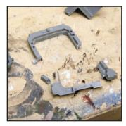
Step 5 - Isolate breaks, make neater cuts: Making cuts that are easy to fix allows us to extend the shrunken frame to fit the sponson properly.
