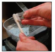
**Resin:** Resin parts should also be scrubbed. An all-purpose cleaner works well.
