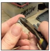
Step 3 - Remove Lugs: With a pair of clippers, remove the triangular lugs from the weapon mount.
