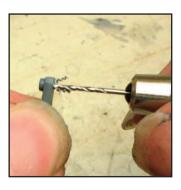
Step 9 - Pilot hole: Very carefully, we drill a pilot hole to a depth of about half the thickness of the post. To retain strength, it is important not to drill right through.
