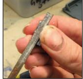
Step 4 - File Flat: Using a flat file, ensure the mounting surface is smooth.
