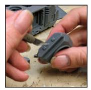
tise Back of Turret: Mark and drill a hole for a magnet on the back of the turret. Bore out witha 4.5mm bit and install a magnet.
