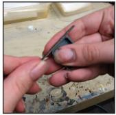
**File:** The leftover nub on the part can be filed away using a needle file.
