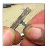
Step 11 - File flat: Filina across the hole with a flat file, smooth the hole out so there is a 1 mm clearance so the maanet can be fitted flush with the post.
