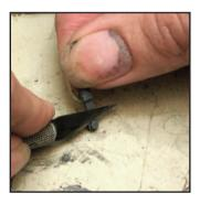
Step 7 - Trim axle: First we remove the axle from the outer side of the mounting post. Ensure everything is removed so the post is flat and smooth.
