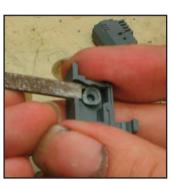
Step 13(b) - File down: If the mounting post aets cauaht on the slot or on the bored-out parts of the guns, further filina down is needed.
