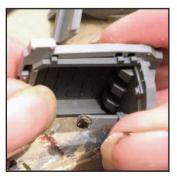
Step 4(a) - Prepare for the Worst: This part has shrunk badly. The best way to fit it is to make a number of controlled cuts. Forcing it...
